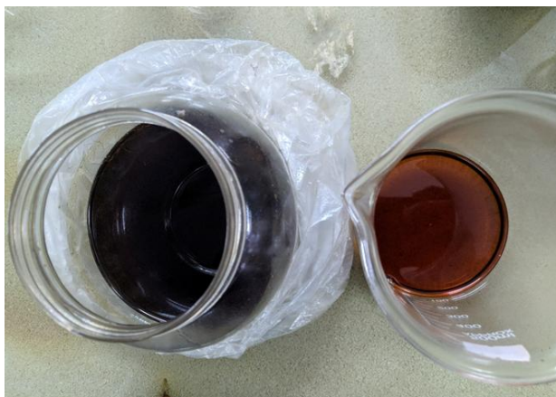
Figure 3. 4: Neem oil (Left) and produced bio diesel from this neem oil (Right)
